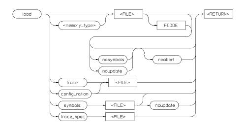
This command transfers absolute files from the host computer into emulation or target system RAM. With other parameters, the load command can load emulator configuration files, trace records, trace specifications, or symbol files.
