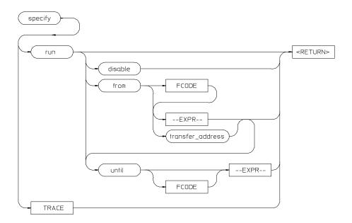
This command prepares a **run** or **trace** command for execution, and is used with the **cmb\_execute** command.
