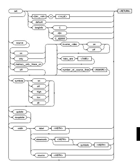
Controls the display format for the data, memory, register, software breakpoint, and trace displays. With the **set** command, you can adjust the display format results for
