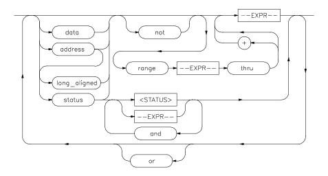
The **QUALIFIER** parameter is used with **trace only**, **trace prestore**, **TRIGGER**, and **trace counting** to specify states captured during the trace measurement.
