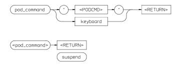
Allows you to control the emulator through the direct HP 64700 Terminal Interface.
