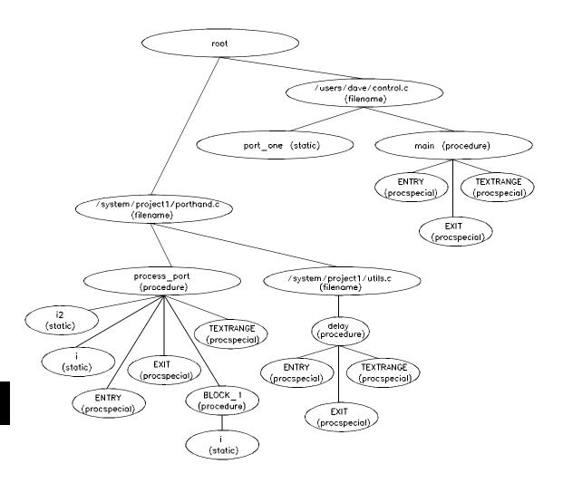
Note that SRU does not build tree nodes for variables that are dynamically allocated on the stack at run-time, such as i and j within the delay () procedure.
