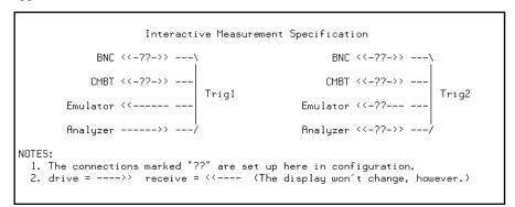
This display illustrates the possible connections between the internal lines (trig1 and trig2) and the emulator, analyzer, and external devices.
