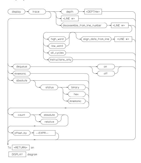
This command displays the contents of the trace buffer.
