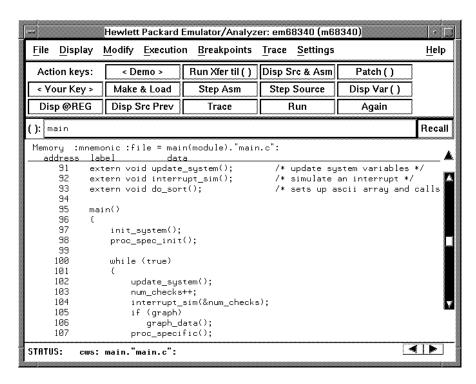
The default display mode settings cause source lines and symbols to appear in displays where appropriate. Notice you can use symbols when specifying expressions. The global symbol "main" is used in the command above to specify the starting address of the memory to be displayed.
