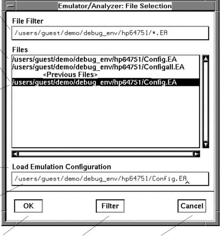
Clicking this button chooses the file name displayed in the text entry area and closes the dialog box. Entering a new file filter and clicking this button causes a list of files matching the new filter to be read from the directory. Clicking this button cancels the file selection operation and closes the dialog box.
