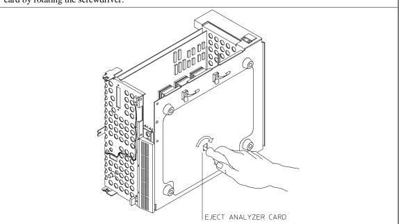
Do not remove the system control board. This board is used in all HP 64700 emulation and analysis systems.
